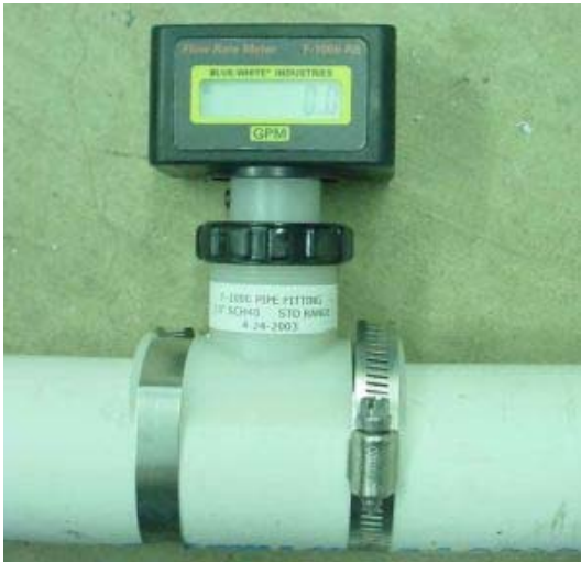
Figure-6 Digital Water-Flow Adjustment Manifold
